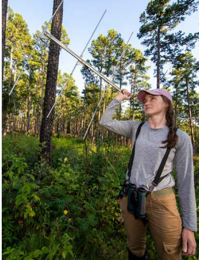
Kristen Heath-Acre scans for tagged brown-headed nuthatches using a very high frequency (VHF) radio antenna in the Missouri Ozarks.
