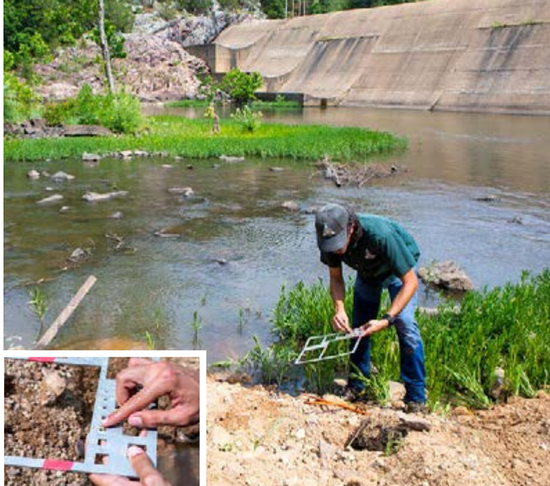
MDC researcher Anthony Cole samples rocks in gravel placed along the riverbank below the Taum Sauk Dam to determine sizes and distribution.
