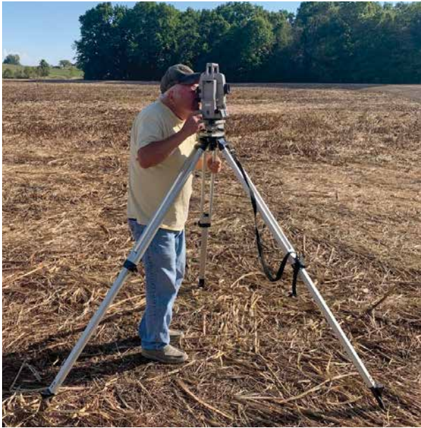
Figure 21a: A surveyor using a total station.
