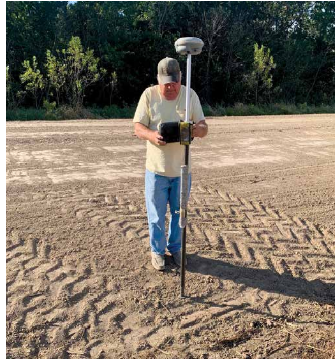
Figure 22b: A surveyor taking shots with survey grade GPS unit that is mounted to a rod or pole.
