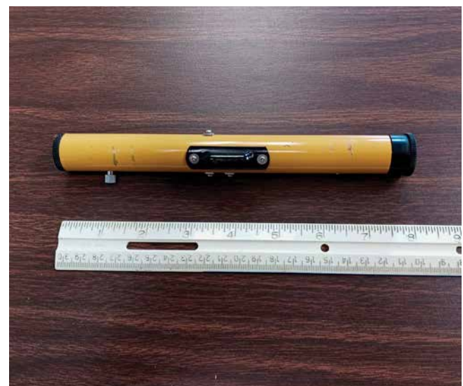
Figure 16: Hand levels, like the one shown here, are handy for general survey information but are not typically used to obtain data for design purposes.
