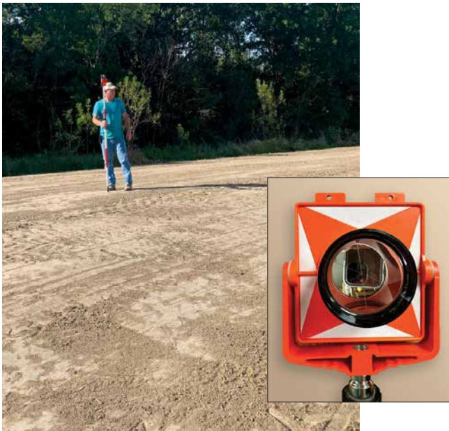
Figure 21b: A prism, or target, is attached to a rod and used to accept signals sent by the total station.
