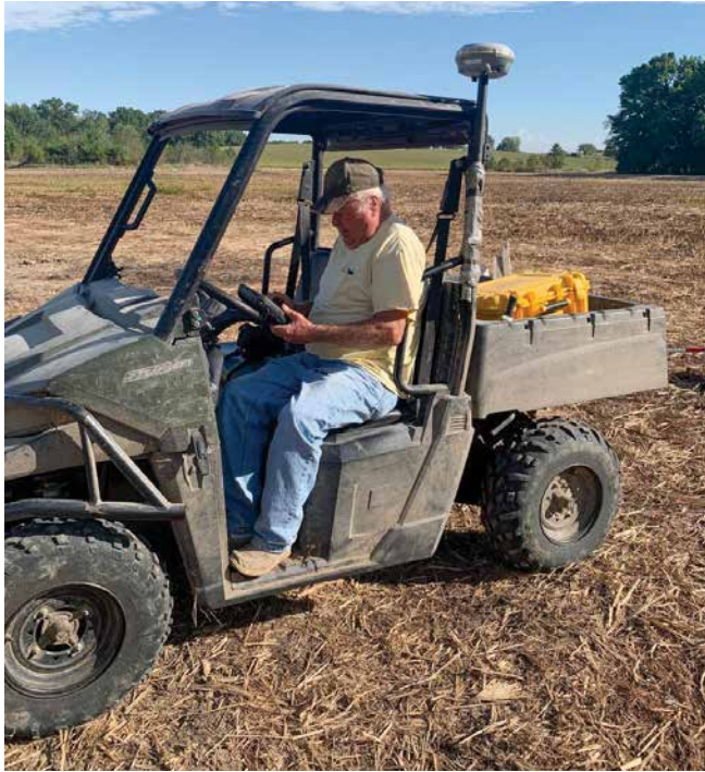
Figure 22a: Surveying with a survey grade GPS unit mounted to a UTV.
