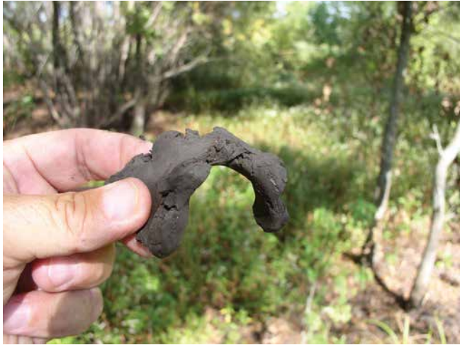
Figure 8: A soil ribbon made from a sample taken in the field. The 2" plus length indicates greater than 25% clay.
