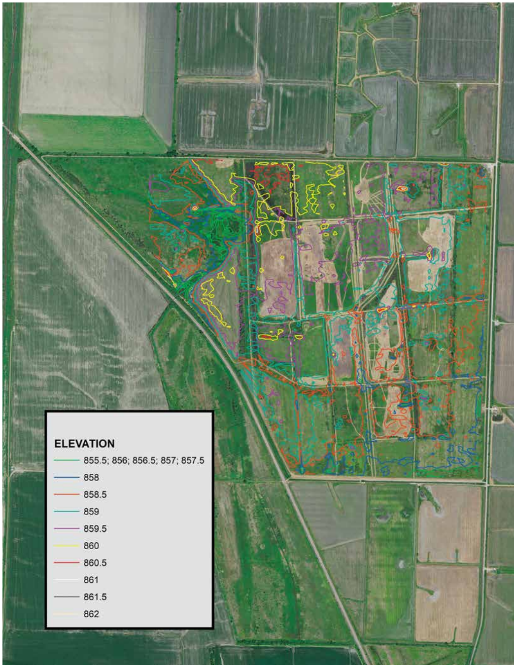
Figure 23: GIS-formatted survey completed using survey grade GPS. In this example, each contour line (elevation) has been assigned a color to help the user visualize “depth” or changes in topography.
