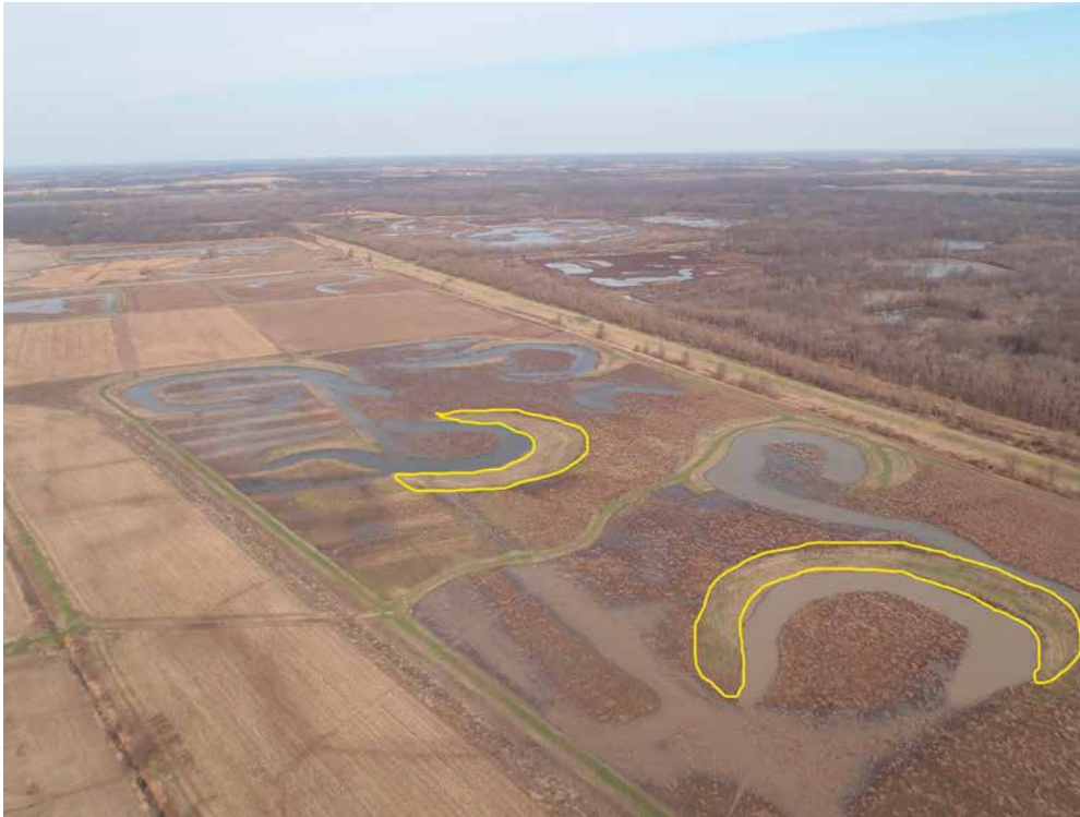
Figure 27: Aerial view of a spoil. The area outlined in yellow shows the spoil. Note how the spoil blends into natural ground features.
