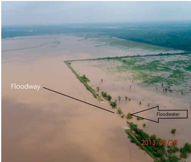
Figure 28a: A constructed floodway created by downgrading an existing flood protection levee.
