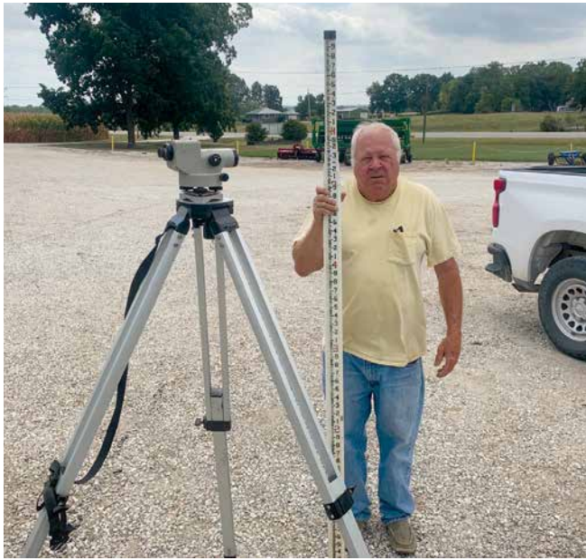
Figure 19: A dumpy level and survey rod.
