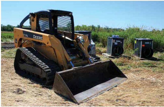
Figure 50: A skid-steer loader can be a very handy piece of equipment for wetland restorations; however, its capabilities are limited by its size.
