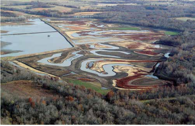
Figure 31a: Creative borrow is a construction method where fill material is taken from areas that resemble naturally occurring features that occur on the landscape, such as the oxbow lakes shown here.
