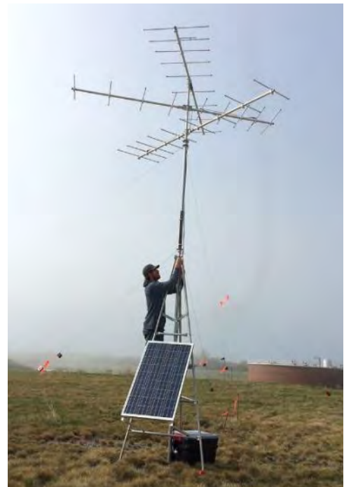
A free-standing Motus station powered by solar. Motus.org
