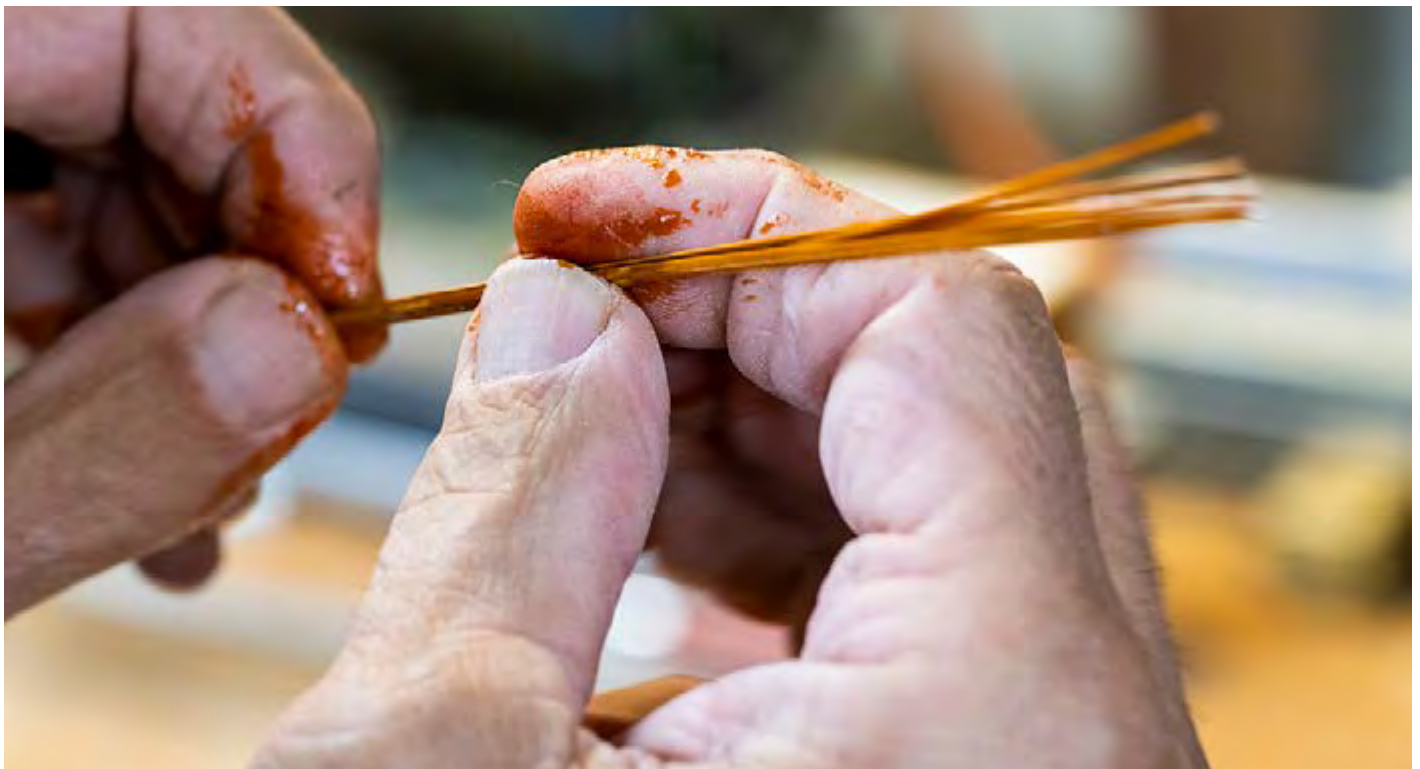
Top: Triangular strips are planed on a hand mill. Bottom: Six tapered strips are glued together.
