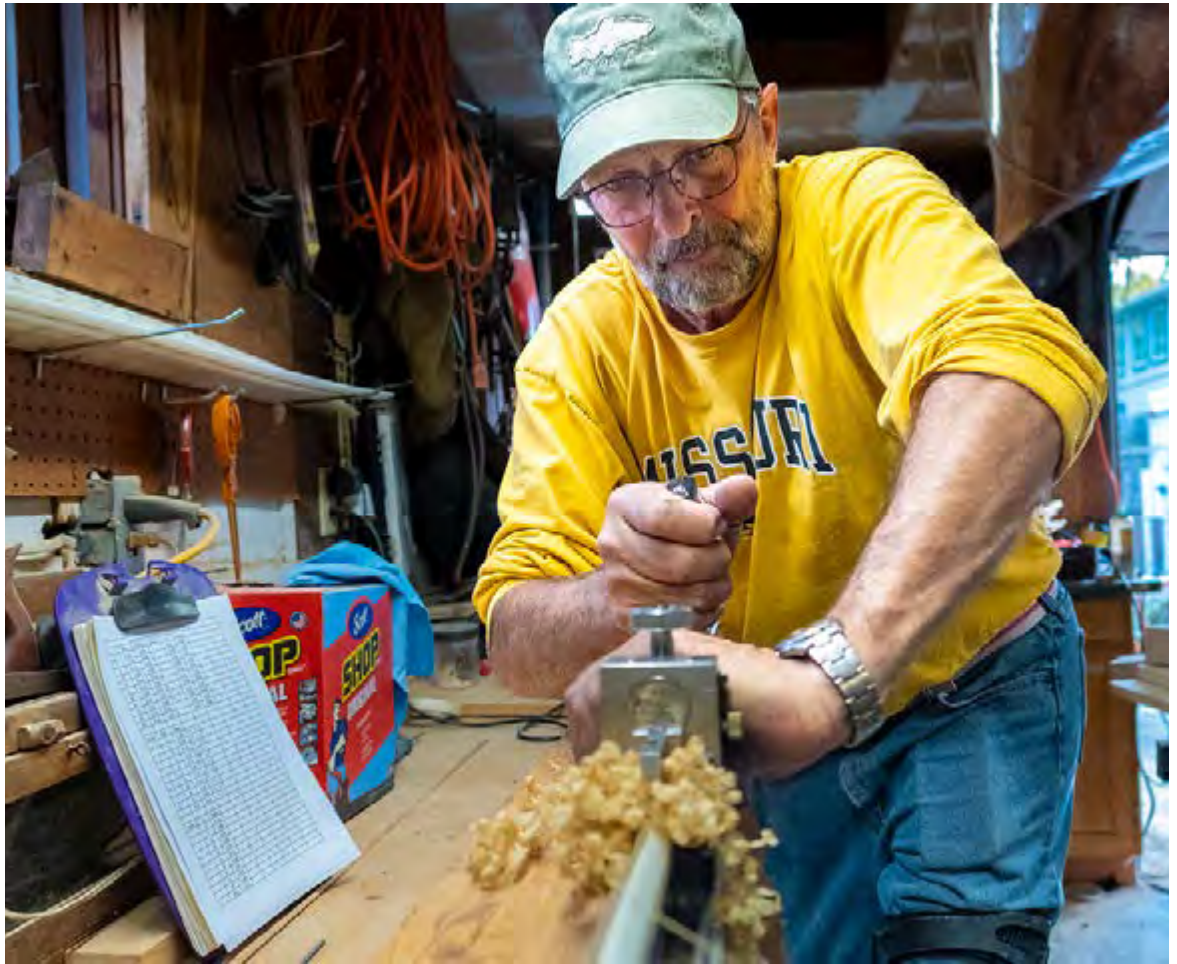
Top: Triangular strips are planed on a hand mill. Bottom: Six tapered strips are glued together.
