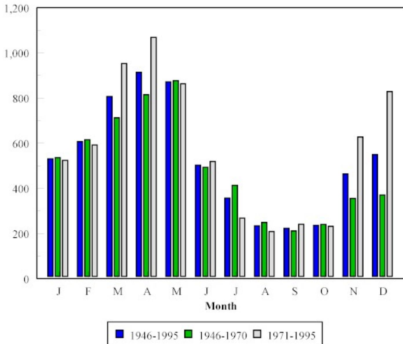
Figure Hy07. Flow duration changes between two time periods for Station 07057500 (North Fork near Tecumseh) (USGS 1999e).
