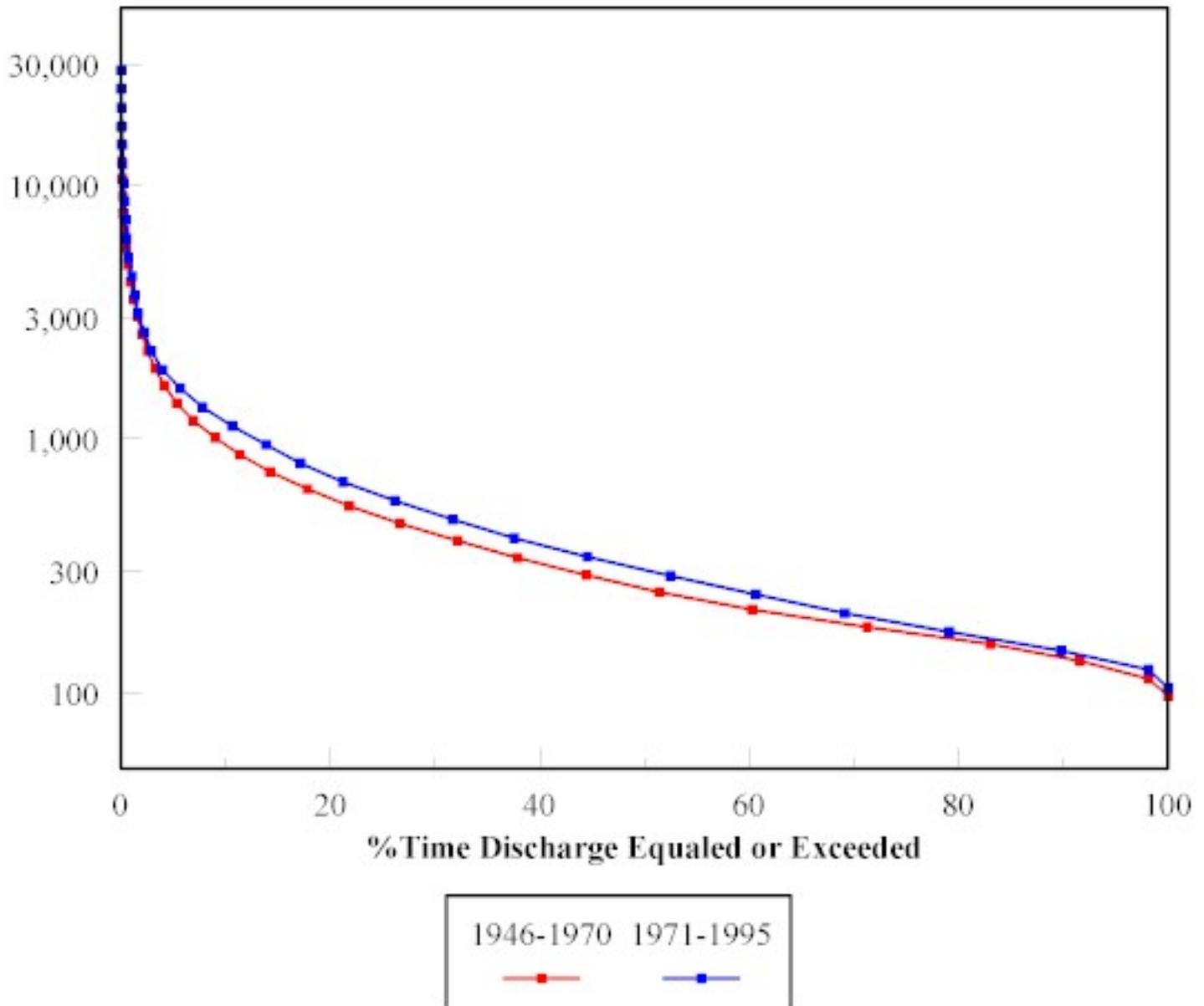
Figure Hy09. Comparison of flow duration for Station 07057500 (North Fork River near Tecumseh) and Station 07058000 (Bryant Creek near Tecumseh) (USGS1999e).
