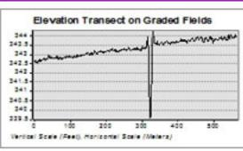
Elevations range from 344 - 342.5 ft. across the field and dips down to 339.5 at the ditch. It is a much flatter surface.
